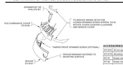
VIEW SHOWING REMOVAL OF COVER (SAME PROCEDURE WITH OR W/O SPACER)
